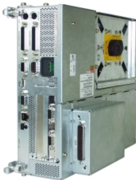
Fig. 3-4 PCU 50 with MCI-Board Extension, external variant
