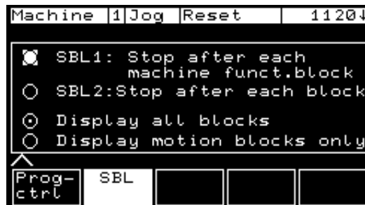
Fig. 3-7 Program control – Single block
