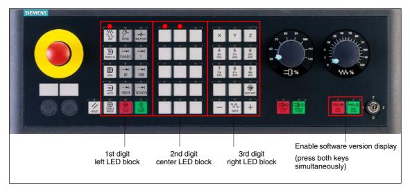
Fig. 8-18 MCP software version display
