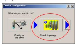
Compare the DRIVE-CliQ topology displayed in the STARTER with the topology of the drive unit.
