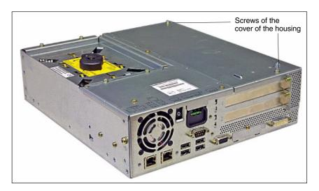
Fig. 2-8 Cover of the housing of the PCU 50.3
