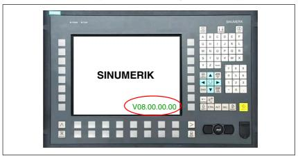
Fig. 5-2 Display in the SINUMERIK 840Di sl startup image
