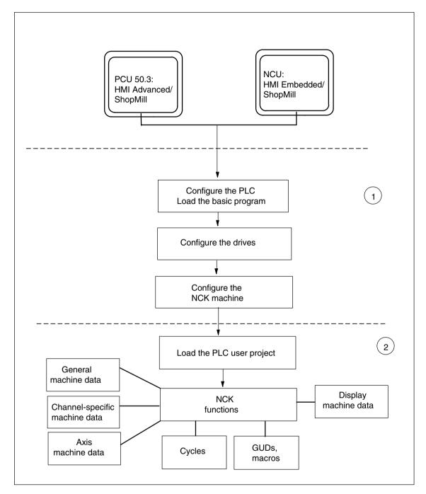
Fig. 4-1 General sequence of initial startup
