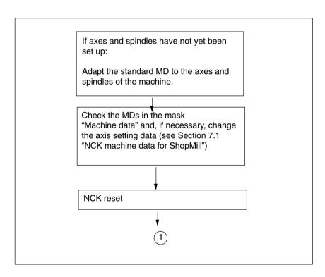
Fig. 4-3 NC SINUMERIK 840D sl installation and startup
