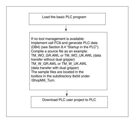
Fig. 4-2 PLC installation and startup
