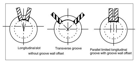
Fig. 9-1 Grooves with and without groove wall offset
