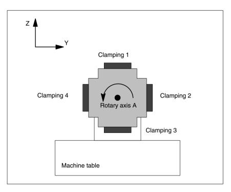
Fig. 9-3 Rotating clamping device (reversible clamping device)
