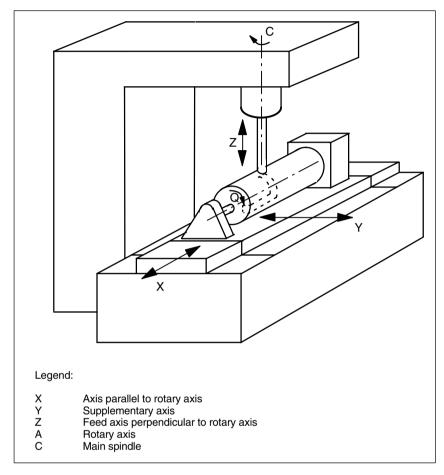
Fig. 9-2 Machining grooves on a cylinder surface with X-C-Z kinematics
