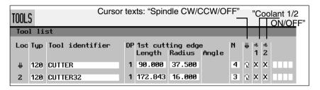
Fig. 8-3 Tool list: Coolant and direction of spindle rotation
