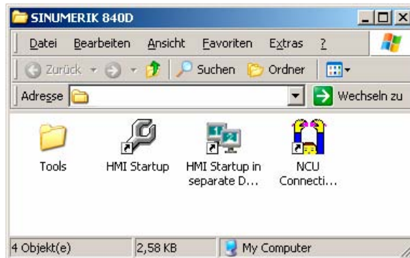
Fig. 4-2: Linking to the desktop switching application
