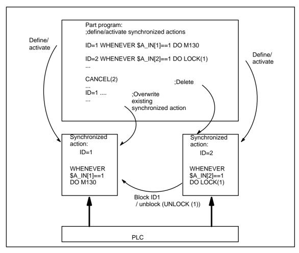
Fig. 2-10 Setting up/locking modal synchronized actions/deleting
