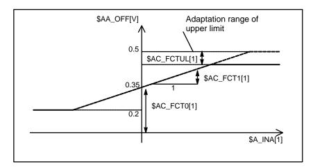
Fig. 6-1 Clearance control with variable upper limit
