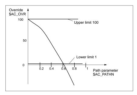
Fig. 6-3 Regulate velocity continuously
