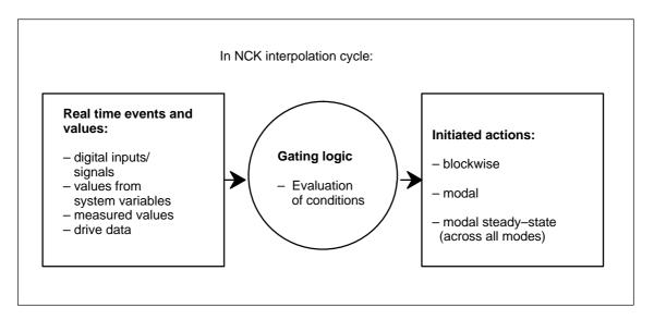
Fig. 1-1 Schematic diagram of synchronized actions
