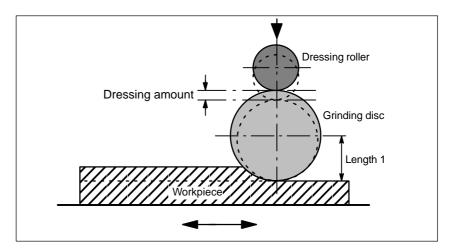
Fig. 2-8 Dressing during machining using a dressing roller
