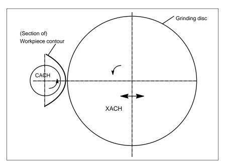
Fig. 6-5 Diagrammatic representation of non-circular contour grinding
