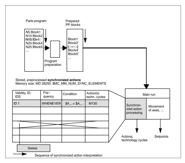
Fig. 2-1 Schematic diagram illustrating processing of synchronized actions
