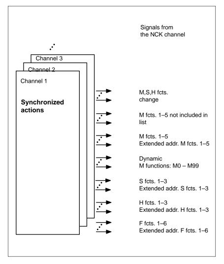
Fig. 5-1 PLC interface signals for synchronized actions
