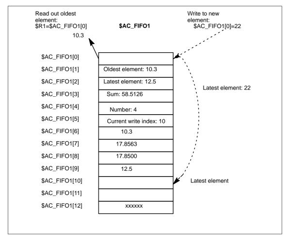
Fig. 2-3 Example of FIFO variables
