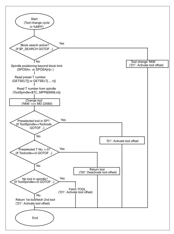
Fig. 6-7 Flowchart for tool-changing cycle
