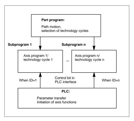
Fig. 2-11 Axis programs/technology cycles
