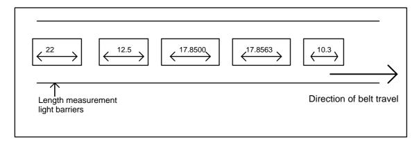
Fig. 2-2 Product lengths of sequence of parts on conveyor belt
