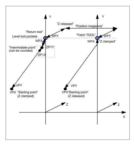
Fig. 6-6 Schematic sequence for tool-changing cycle
