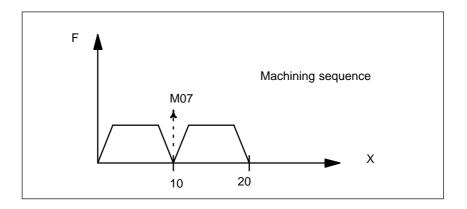
Solution with synchronized action: 1 set N10 WHEN \$AA\_IM[X] >= 10 DO M07 N20 G1 X20 F150
