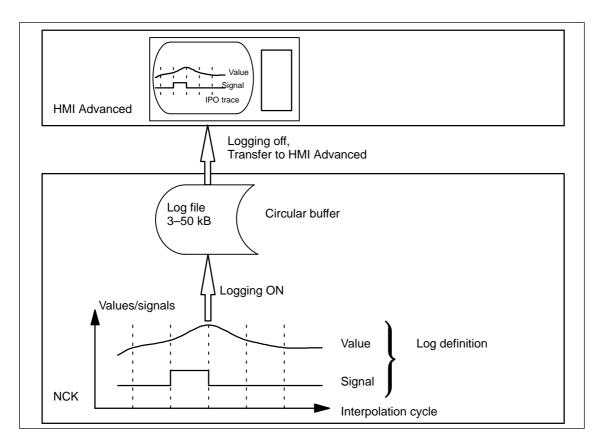
Fig. 2-13 Schematic representation of Log real-time variables process
