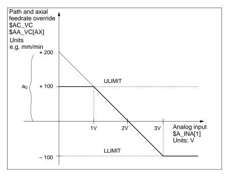
Fig. 6-2 Diagram illustrating adaptive control
