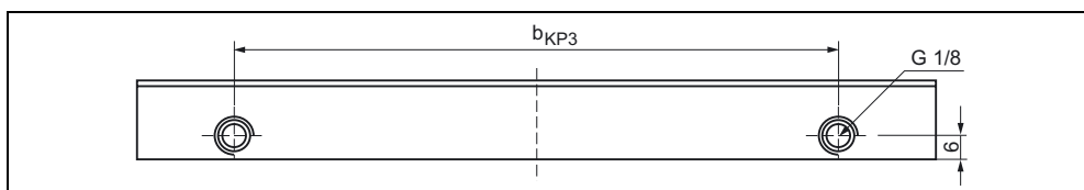
Figure 13-12 Connector layout of the secondary section cooling with combi adapter (face view)
