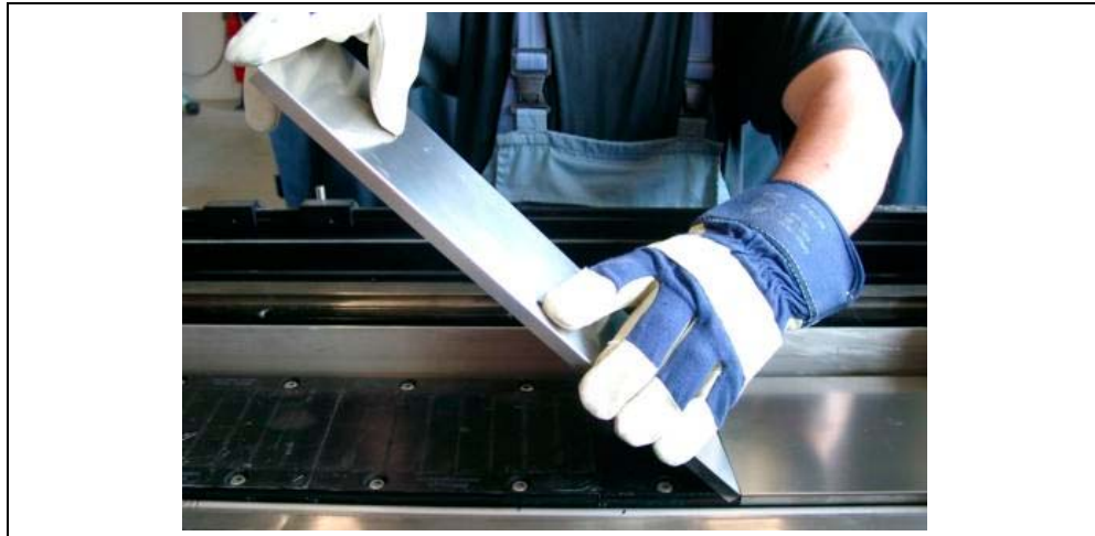
Figure 13-26 Mounting another segment of a segmented secondary section cover
