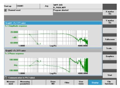
Figure 11-6 Optimized speed control loop
