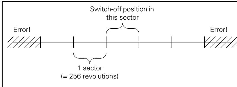
When the motor is switched on and to the switch-off position two complete sectors are in between (further than the sector "after next"), the error message Switch-off pos. <axis> unequal ENDAT is immediately displayed after the drives are switched on.
