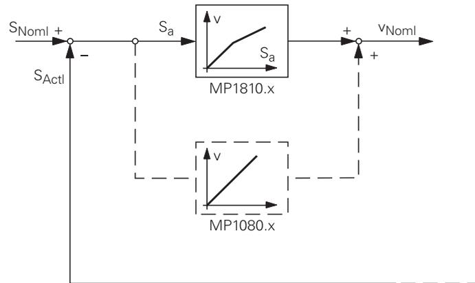
The nominal position value  $s_{noml}$  for a given axis is compared with the actual position value  $s_{actl}$  and the resulting difference is the following error  $s_a$ :
