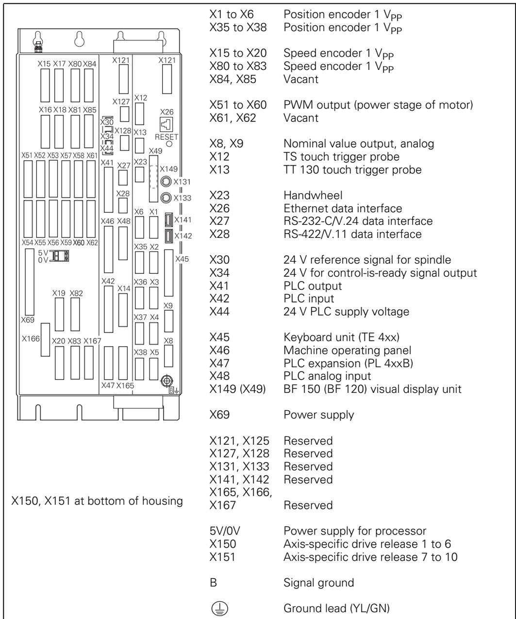
**MC 422B with 5 position encoder inputs and CC 422 with 6 control loops**
