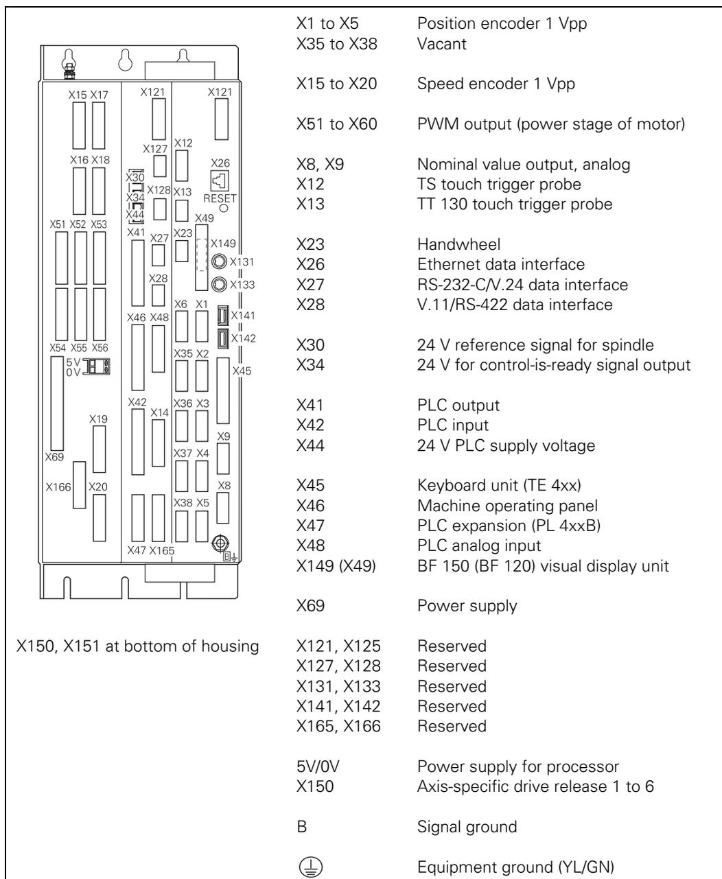
**MC 422 M with 10 position encoder inputs and CC 422 with 10 control loops**
