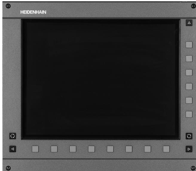
One of the two flat-panel displays are connected to the iTNC 530:
