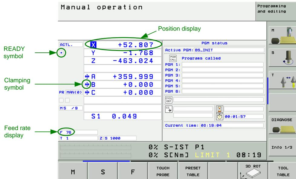
To operate with axes or spindles the appropriate enables are required.
