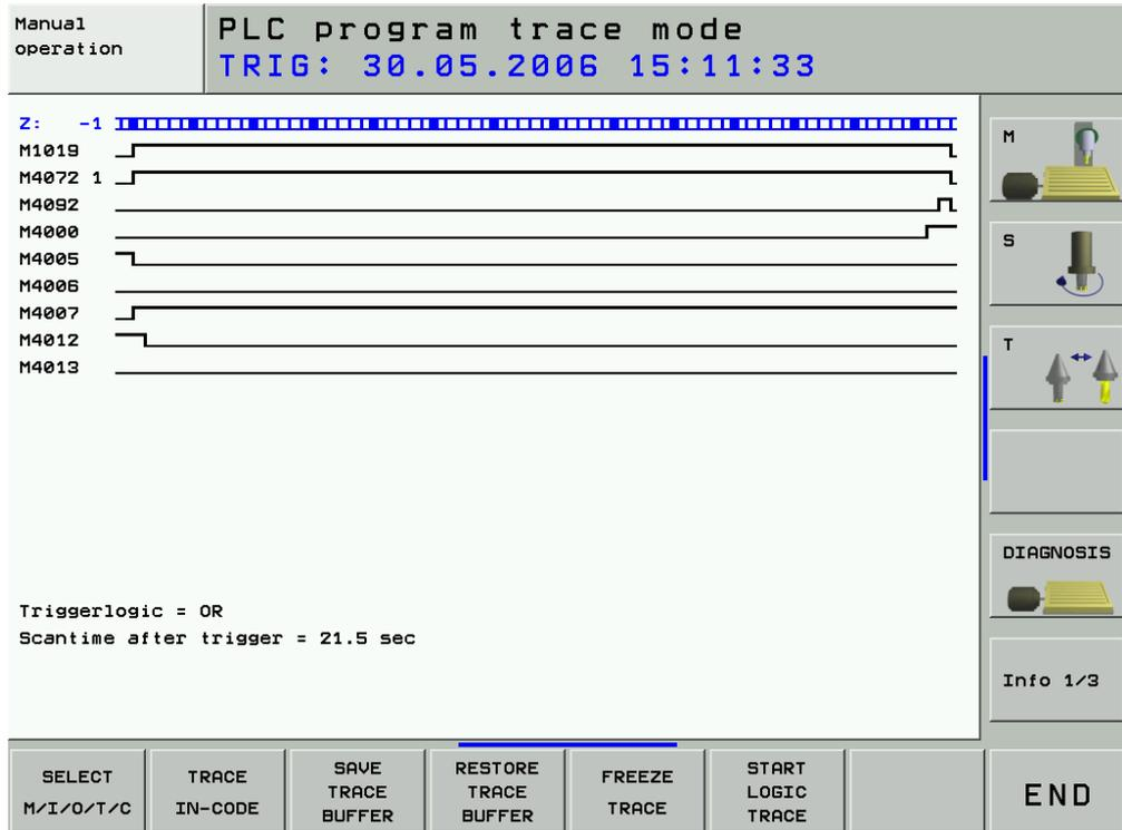
The trigger event is displayed on the left edge of the display with the PLC run 0. It is possible to scroll -512 PLC cycles to the left and +512 PLC cycles to the right.
