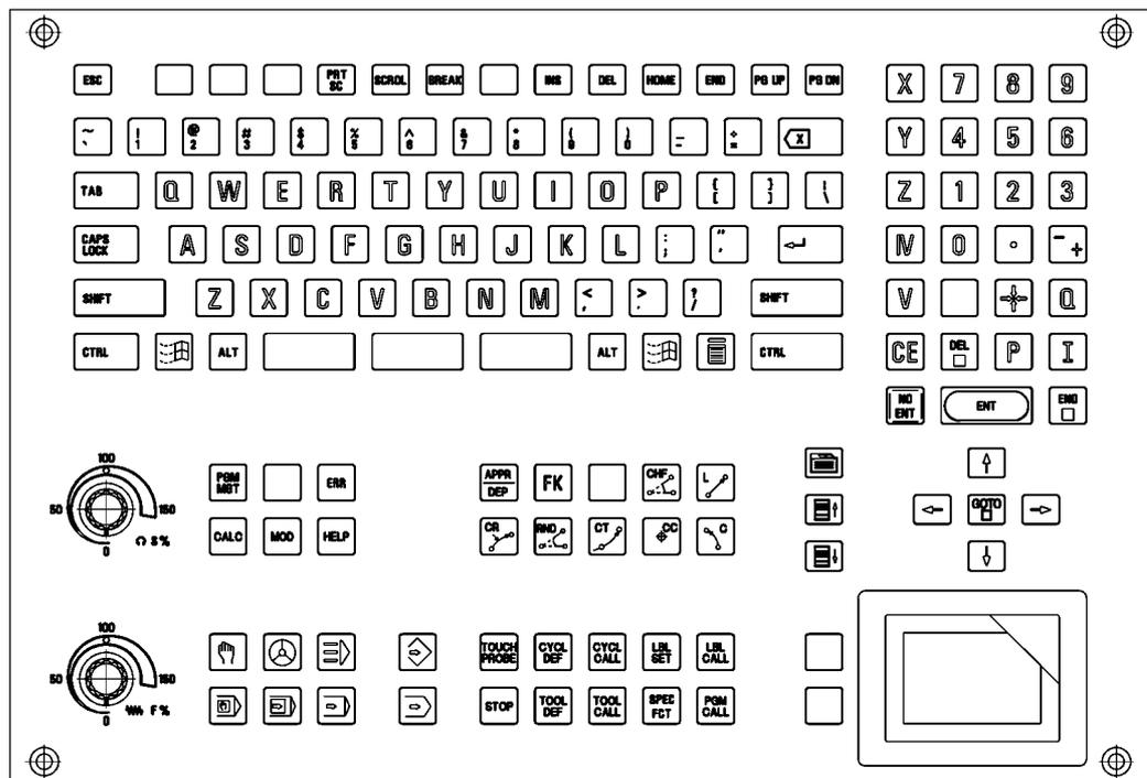
TE 520 B (with additional smarT.NC keys, without mouse pad)
