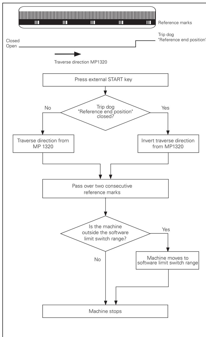
If during automatic referencing the trip dog is not closed until it is in the reference end position range, the contouring control will ignore this signal. It is therefore necessary that there are at least two reference marks in the range of the reference end position.
