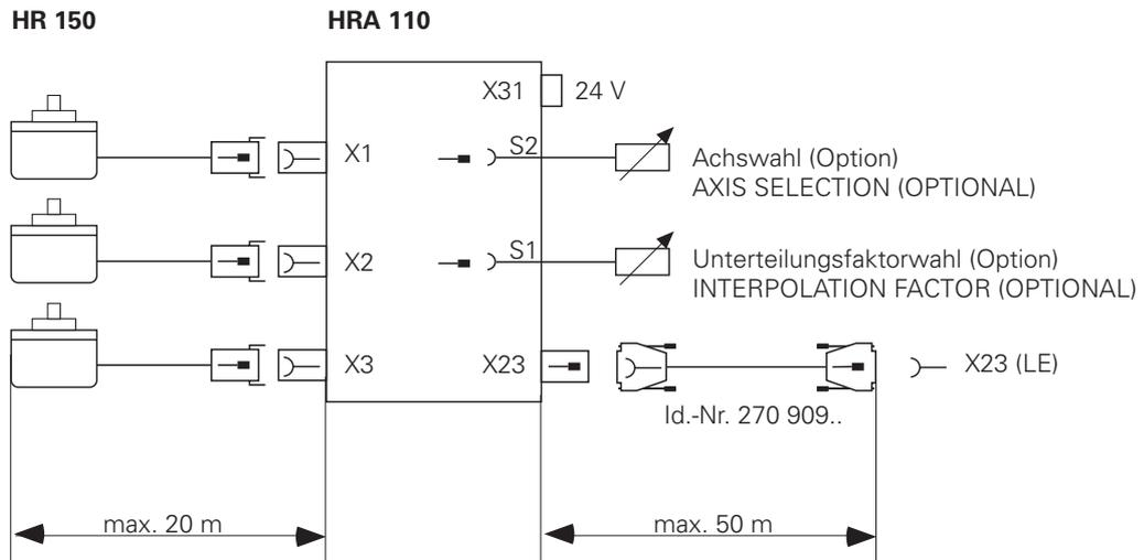
An additional switch enables you to select, for example, the interpolation factor for the handwheel. The current position of the step switch is evaluated by the PLC.
