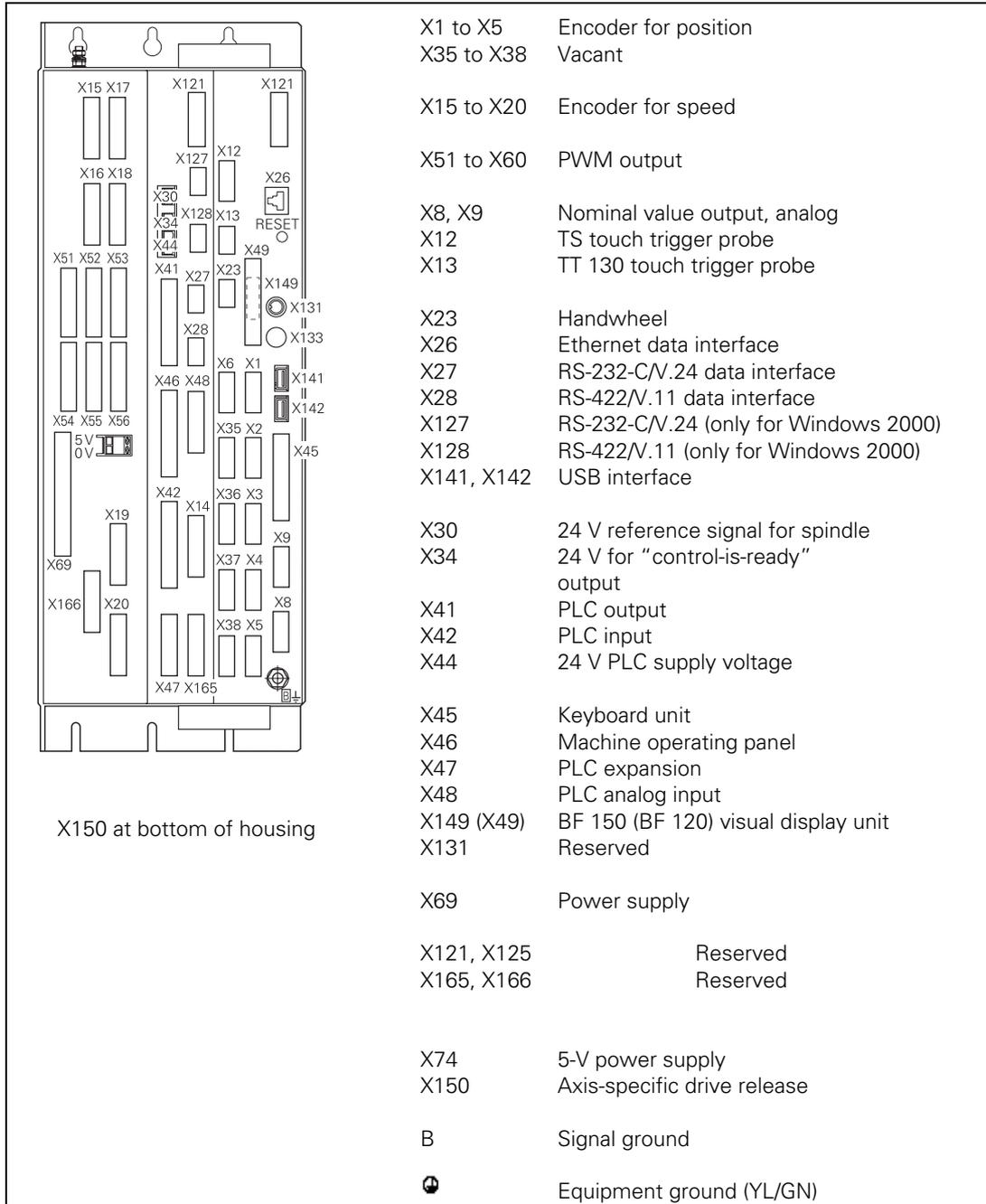
**MC 422B with 10 position encoder inputs and CC 422 with 10 or 12 control loops**
