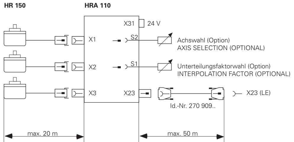
An additional switch enables you to select, for example, the interpolation factor for the handwheel. The current position of the step switch is evaluated by the PLC.
