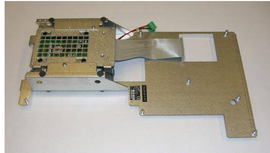
Removal and insertion of the HDR, shipping brace
