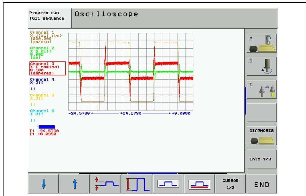
During recording, the trains of selected signals are constantly depicted. After recording ends, the memory contents are displayed. For every channel, the manner of the signal and the resolution are also shown. The length of the recorded range referenced to the entire memory contents is displayed as a bar in the status field.
