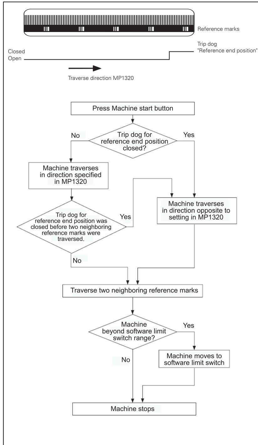
Function when MP1350.x = 0. This setting is used only to ensure compatibility. Do not use for new installations.
