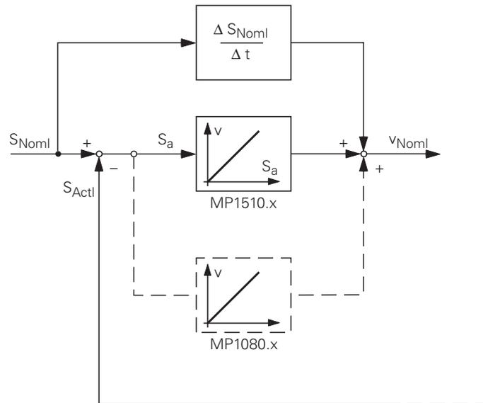
Unlike operation with following error, the optimum kv factor for each axis when operating with interpolated axes is set by the machine manufacturer.
