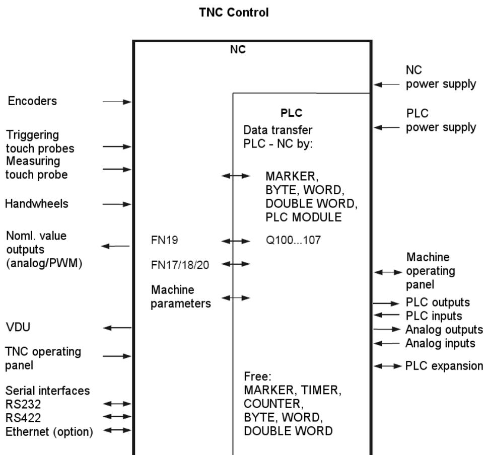
Depending on the type of control, various inputs and outputs are available for the data exchange with the machine.
