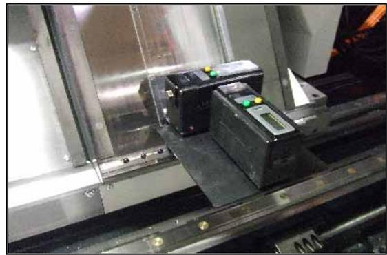
The Z-axial level is measured.
