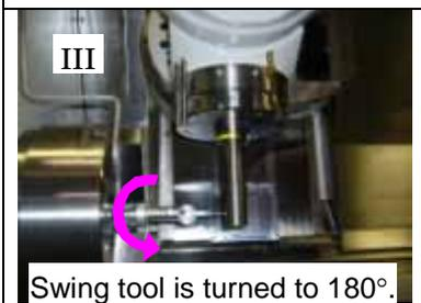
(2) Adjustment of RS12 (Measurement is carried out on the 2nd spindle under the condition of the Y-axis compensated and the B-axis at  $90^\circ$ .)
