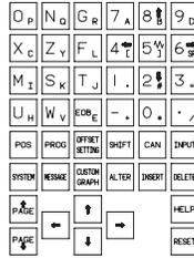
Fig. 1.1 (c) MDI Keyboard of 9" Small CRT/MDI Panel or 8.4" Small LCD/MDI Panel
