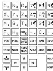
Fig. 1.1 (g) MDI Keyboard of 9" Small CRT/MDI Panel or 8.4" Small LCD/MDI Panel
