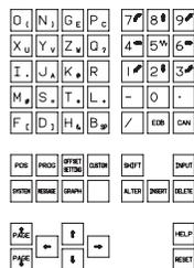
Fig. 1.1 (h) MDI Keyboard of 9.5" LCD/MDI Panel (Horizontal)
